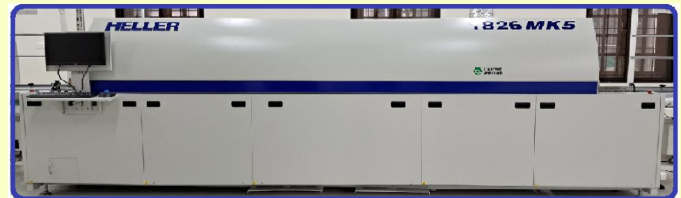
Reflow Oven (RO) HELLER 1826 MK5
